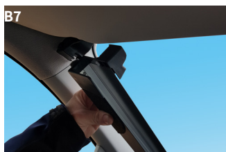
B7: Carefully fold the guides over the handle bar until it is fully down. Do not touch the guide except in the areas marked with felt, as the metal parts may be hot.
