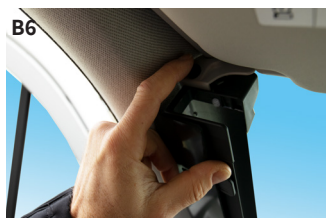
B6: Now release the latching of the guide one after the other by pressing the key.
